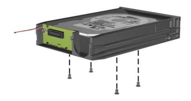
Slide the hard drive back to disconnect it from the carrier then lift it up and out of the carrier.
